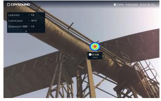
A coal chemical enterprise detected a gas leak in an overhead pipeline using the CRY8125 Ex Acoustic Imaging Camera, which could not be identified by traditional methods.
